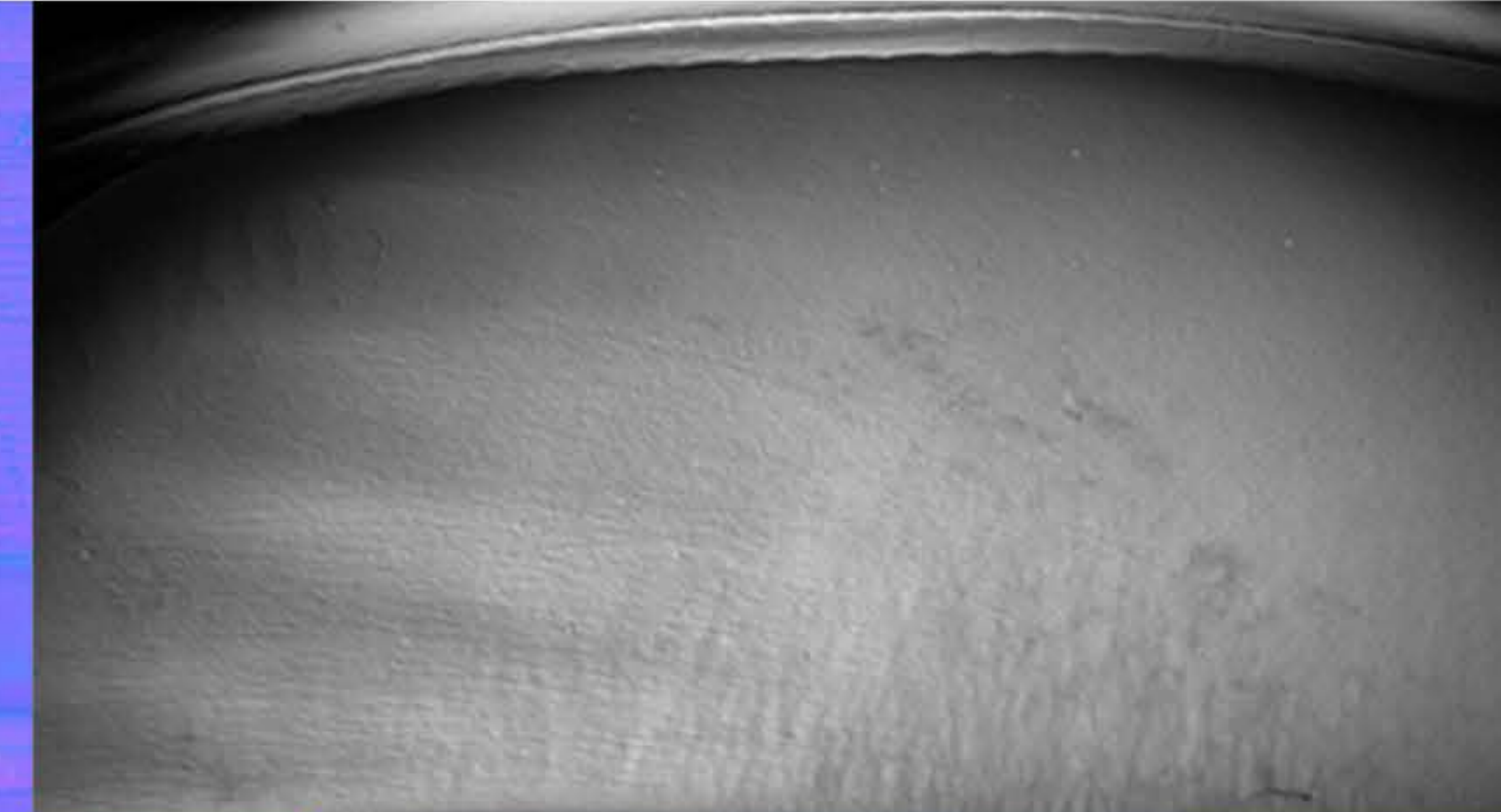
Inspection of pin head. Scratches
