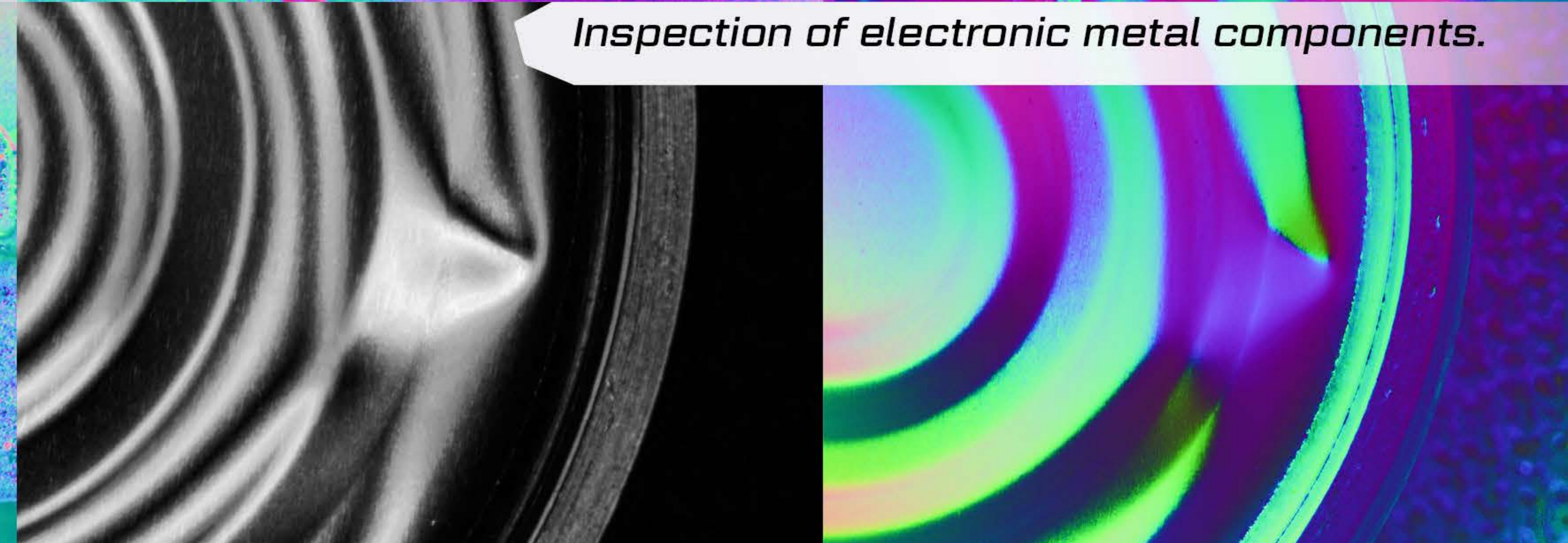
Inspection of electronic components. Contamination/Uneven Coverage
